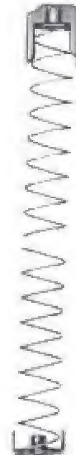
Fig. 18 Follower, with follower spring and locking plate
